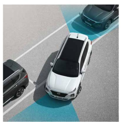
Parking Distance Warning (PDW) (Optional) Sensors in the front and rear bumpers detect and warn the driver about imminent obstacles for safe parking.
