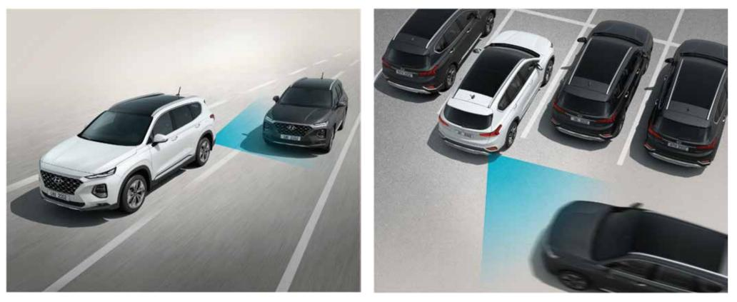
Blind-Spot Collision Warning (BCW) (Optional) Radar sensors in the rear bumper are used to warn the driver of approaching vehicles in the blind spot area.
