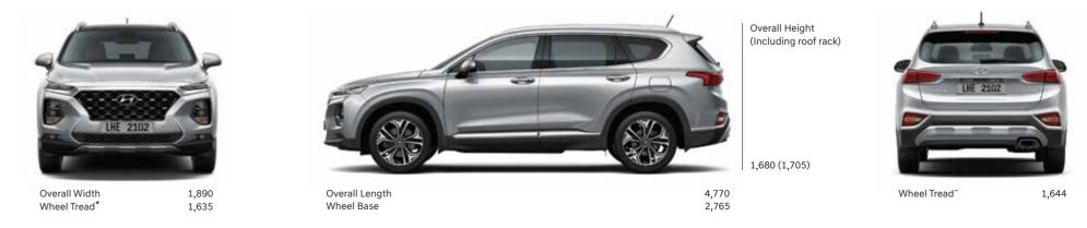
Unit : mm \*Wheel Tread • 17" Alloy Wheel (Front / Rear) : 1,643 / 1,652 • 18" Alloy Wheel (Front / Rear) : 1,638 / 1,647 • 19" Alloy Wheel, Dark Hypersilver Wheel (Front / Rear) : 1,643 / 1,647
