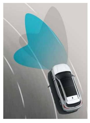
Low Beam Assist-Dynamic (LBA-D) (Optional) The headlamps respond to the turn of the steering wheel and illuminate the part of the road the driver is turning towards.
